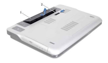
1 battery 2 battery release latch
